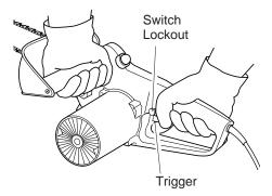
Figure 9 - Switch Lockout and Trigger Location
